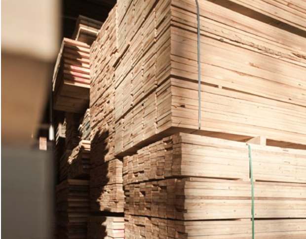
PEFC/06-34-110 or FSC® C119602 - certified lamellae undergo machine strength grading and are sorted according to surface quality
